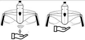
Bring your hand towards the sensor up to 2 cm and maintain this distance until the desired light intensity is reached Acoustic signal: 1 beep at command Maximum intensity reached: 2 beeps Minimum intensity reached: 1 beep
