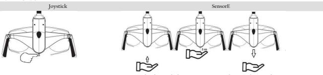
Press right or left and release Acoustic signal: I beep
