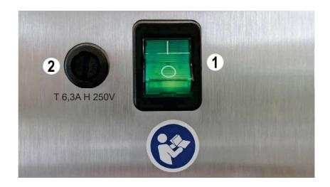
The treatment unit is equipped with a power switch ① on the chair base. The power switch connects the treatment unit with the power supply.
